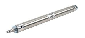
NITRA pneumatic cylinder, non-repairable, 1-1/4in bore, 7/16in rod diameter, 10in stroke, double acting, magnetic piston, double end mount.
