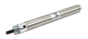
NITRA pneumatic cylinder, non-repairable, 1-1/4in bore, 7/16in rod diameter, 8in stroke, double acting, front nose mount.
