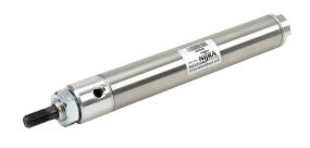
NITRA pneumatic cylinder, non-repairable, 1-1/4in bore, 7/16in rod diameter, 6in stroke, double acting, front nose mount.
