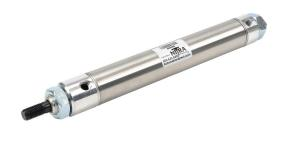
NITRA pneumatic cylinder, non-repairable, 1-1/4in bore, 7/16in rod diameter, 6in stroke, double acting, double end mount.
