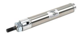
NITRA pneumatic cylinder, non-repairable, 1-1/4in bore, 7/16in rod diameter, 5in stroke, double acting, front nose mount.
