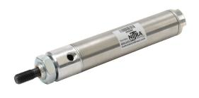
NITRA pneumatic cylinder, non-repairable, 1-1/4in bore, 7/16in rod diameter, 4in stroke, double acting, front nose mount.
