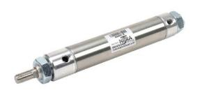
NITRA pneumatic cylinder, non-repairable, 1-1/4in bore, 7/16in rod diameter, 4in stroke, double acting, magnetic piston, double end mount.
