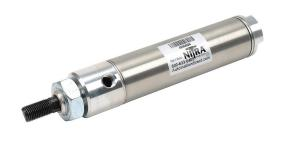
NITRA pneumatic cylinder, non-repairable, 1-1/4in bore, 7/16in rod diameter, 3in stroke, double acting, front nose mount.
