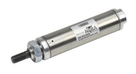
NITRA pneumatic cylinder, non-repairable, 1-1/4in bore, 7/16in rod diameter, 2in stroke, single acting, front nose mount.
