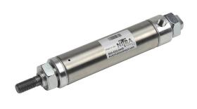
NITRA pneumatic cylinder, non-repairable, 1-1/4in bore, 7/16in rod diameter, 2in stroke, single acting, double end mount.
