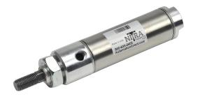
NITRA pneumatic cylinder, non-repairable, 1-1/4in bore, 7/16in rod diameter, 2in stroke, double acting, front nose mount.
