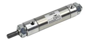
NITRA pneumatic cylinder, non-repairable, 1-1/4in bore, 7/16in rod diameter, 2in stroke, double acting, double end mount.
