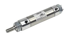
NITRA pneumatic cylinder, non-repairable, 1-1/4in bore, 7/16in rod diameter, 2in stroke, double acting, magnetic piston, double end mount.
