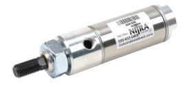
NITRA pneumatic cylinder, non-repairable, 1-1/4in bore, 7/16in rod diameter, 1in stroke, double acting, front nose mount.
