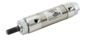
NITRA pneumatic cylinder, non-repairable, 1-1/4in bore, 7/16in rod diameter, 1in stroke, double acting, double end mount.
