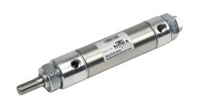
NITRA pneumatic cylinder, non-repairable, 1-1/4in bore, 7/16in rod diameter, 1in stroke, double acting, magnetic piston, double end mount.
