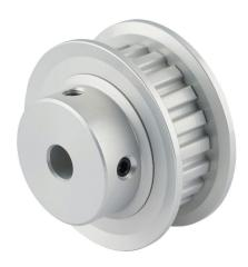
Sung-II Machinery timing pulley, aluminum, 1/5in XL pitch, 20 tooth, 1.273in pitch diameter, 1/4in bore, hub with flanges. For use with 3/8in wide belt.
