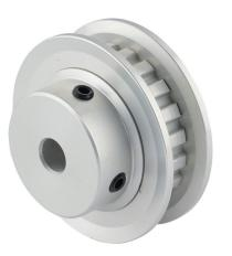
Sung-Il Machinery timing pulley, aluminum, 1/5in XL pitch, 20 tooth, 1.273in pitch diameter, 1/4in bore, hub with flanges. For use with 1/4in wide belt.
