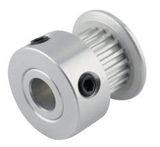
Sung-Il Machinery timing pulley, aluminum, 0.08in MXL pitch, 20 tooth, 0.509in pitch diameter, 1/4in bore, oversize hub with flange. For use with 1/4in wide belt.
