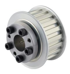
Sung-Il Machinery timing pulley, aluminum, 3/8in L pitch, 20 tooth, 2.387in pitch diameter, 3/4in bore, no hub with flanges. For use with 1in wide belt. QD bushing included.
