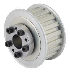
Sung-Il Machinery timing pulley, aluminum, 3/8in L pitch, 20 tooth, 2.387in pitch diameter, 5/8in bore, no hub with flanges. For use with 1in wide belt. QD bushing included.
