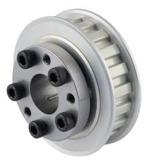
Sung-Il Machinery timing pulley, aluminum, 3/8in L pitch, 20 tooth, 2.387in pitch diameter, 3/4in bore, no hub with flanges. For use with 1/2in wide belt. QD bushing included.
