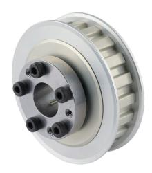
Sung-Il Machinery timing pulley, aluminum, 3/8in L pitch, 20 tooth, 2.387in pitch diameter, 5/8in bore, no hub with flanges. For use with 1/2in wide belt. QD bushing included.
