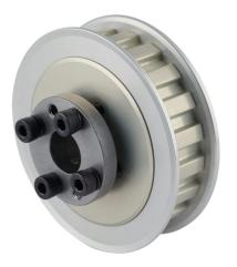
Sung-Il Machinery timing pulley, aluminum, 3/8in L pitch, 20 tooth, 2.387in pitch diameter, 1/2in bore, no hub with flanges. For use with 1/2in wide belt. QD bushing included.
