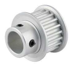
Sung-II Machinery timing pulley, aluminum, 5mm 5M pitch, 20 tooth, 1.253in pitch diameter, 5/8in bore, hub with flanges. For use with 15mm wide belt.
