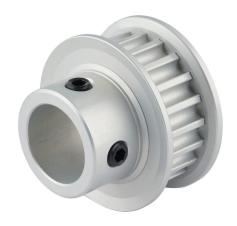
Sung-Il Machinery timing pulley, aluminum, 5mm 5M pitch, 20 tooth, 1.253in pitch diameter, 5/8in bore, hub with flanges. For use with 9mm wide belt.
