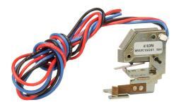
Eaton field installable auxiliary contact, SPDT contact(s), 6A @ 600VAC, 18in pigtail. For use with AutomationDirect (Eaton) 400A frame MCCBs.
