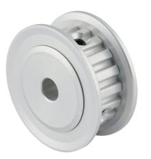
Sung-Il Machinery timing pulley, aluminum, 1/5in XL pitch, 18 tooth, 1.146in pitch diameter, 1/4in bore, no hub with flanges. For use with 3/8in wide belt.
