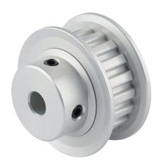
Sung-Il Machinery timing pulley, aluminum, 1/5in XL pitch, 18 tooth, 1.146in pitch diameter, 1/4in bore, hub with flanges. For use with 3/8in wide belt.
