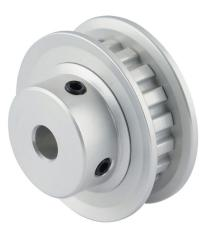
Sung-Il Machinery timing pulley, aluminum, 1/5in XL pitch, 18 tooth, 1.146in pitch diameter, 1/4in bore, hub with flanges. For use with 1/4in wide belt.
