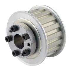
Sung-Il Machinery timing pulley, aluminum, 3/8in L pitch, 18 tooth, 2.149in pitch diameter, 5/8in bore, no hub with flanges. For use with 1in wide belt. QD bushing included.
