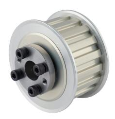
Sung-Il Machinery timing pulley, aluminum, 3/8in L pitch, 18 tooth, 2.149in pitch diameter, 1/2in bore, no hub with flanges. For use with 1in wide belt. QD bushing included.
