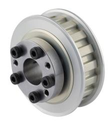
Sung-Il Machinery timing pulley, aluminum, 3/8in L pitch, 18 tooth, 2.149in pitch diameter, 5/8in bore, no hub with flanges. For use with 1/2in wide belt. QD bushing included.
