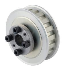
Sung-Il Machinery timing pulley, aluminum, 3/8in L pitch, 18 tooth, 2.149in pitch diameter, 1/2in bore, no hub with flanges. For use with 1/2in wide belt. QD bushing included.
