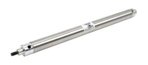
NITRA pneumatic cylinder, non-repairable, 1-1/16in bore, 5/16in rod diameter, 12in stroke, double acting, rear pivot mount.
