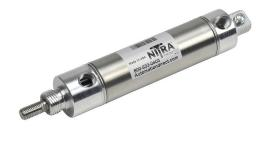
NITRA pneumatic cylinder, non-repairable, 1-1/16in bore, 5/16in rod diameter, 12in stroke, double acting, magnetic piston, rear pivot mount.
