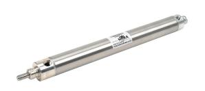
NITRA pneumatic cylinder, non-repairable, 1-1/16in bore, 5/16in rod diameter, 8in stroke, double acting, magnetic piston, rear pivot mount.
