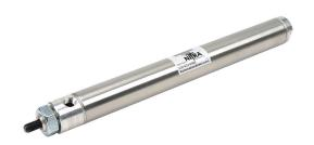
NITRA pneumatic cylinder, non-repairable, 1-1/16in bore, 5/16in rod diameter, 8in stroke, double acting, front nose mount.
