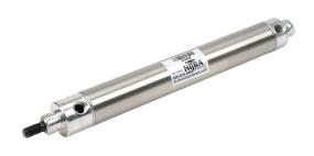
NITRA pneumatic cylinder, non-repairable, 1-1/16in bore, 5/16in rod diameter, 6in stroke, double acting, rear pivot mount.
