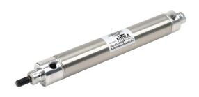
NITRA pneumatic cylinder, non-repairable, 1-1/16in bore, 5/16in rod diameter, 5in stroke, double acting, rear pivot mount.
