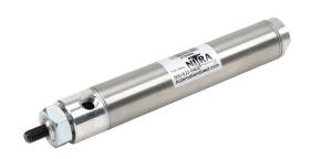
NITRA pneumatic cylinder, non-repairable, 1-1/16in bore, 5/16in rod diameter, 4in stroke, double acting, front nose mount.
