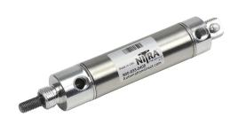
NITRA pneumatic cylinder, non-repairable, 1-1/16in bore, 5/16in rod diameter, 3in stroke, double acting, rear pivot mount.
