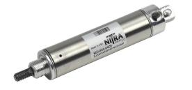
NITRA pneumatic cylinder, non-repairable, 1-1/16in bore, 5/16in rod diameter, 2in stroke, single acting, rear pivot mount.
