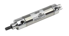
NITRA pneumatic cylinder, non-repairable, 1-1/16in bore, 5/16in rod diameter, 2in stroke, double acting, rear pivot mount.
