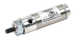
NITRA pneumatic cylinder, non-repairable, 1-1/16in bore, 5/16in rod diameter, 1in stroke, double acting, front nose mount.
