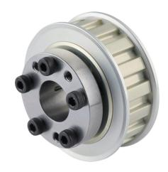
Sung-Il Machinery timing pulley, aluminum, 3/8in L pitch, 17 tooth, 2.029in pitch diameter, 5/8in bore, no hub with flanges. For use with 1/2in wide belt. QD bushing included.
