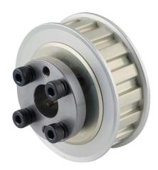
Sung-Il Machinery timing pulley, aluminum, 3/8in L pitch, 17 tooth, 2.029in pitch diameter, 1/2in bore, no hub with flanges. For use with 1/2in wide belt. QD bushing included.
