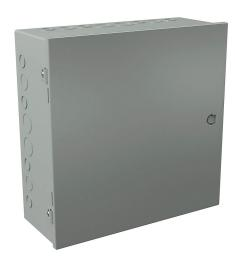
Wiegmann enclosure, NEMA 1, 16 x 16 x 6in (HxWxD), wall mount, with knockouts, carbon steel, ANSI 61 gray, powder coat finish, single-door, integral snap-tight latch.
