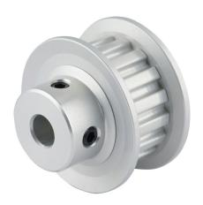
Sung-II Machinery timing pulley, aluminum, 1/5in XL pitch, 16 tooth, 1.019in pitch diameter, 1/4in bore, hub with flanges. For use with 3/8in wide belt.
