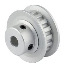
Sung-II Machinery timing pulley, aluminum, 1/5in XL pitch, 16 tooth, 1.019in pitch diameter, 1/4in bore, hub with flanges. For use with 1/4in wide belt.
